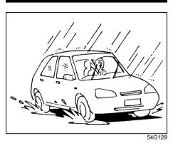
If the wiper blades become brittle or damaged, or make streaks when wiping, replace the wiper blades.
