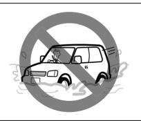
Avoid driving in a flooded area or a deep puddle. If driving in a flooded area is unavoidable, go slowly in the lowest gear. In case that you have driven in a flooded area, stop the vehicle in a safe place while checking the brake effectiveness. Then, ask a SUZUKI dealer or a qualified workshop to check the following inspection items.
