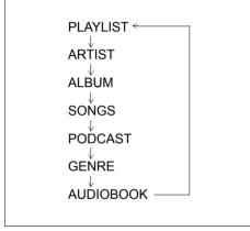
Press "TUNE/FLD PUSH SOUND" knob (2) to select the desired mode.
